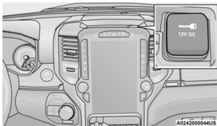
Power Outlet – Top Of Center Stack
