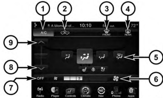
Temperature Controls — Soft-keys
