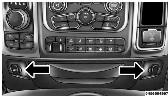
Power Outlets — Center Stack
